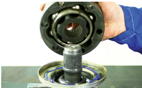
9. Fit CV-joint on shaft, lining up the splines. N.B. Do not forget gasket between inside end cover and CV-joint.
