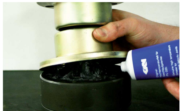
12. Fill inside of CV-joint with approx. half the grease supplied
